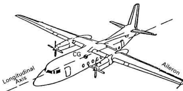
Rolling Rotation about the Longitudinal axis. Control by Ailerons (Lateral control)
